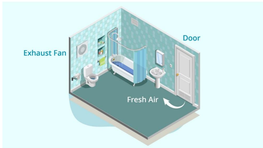
Fresh Air inlet for bathroom
