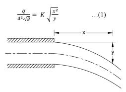
NOTE — It is preferable to avoid any fitting (like flange, coupling) near the end of the pipe; otherwise due correction should be made.
