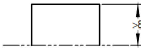
FIG. 4B UNPROTECTED, OVERHANGING SHARP-EDGES (HARD) EQUIPMENT PART
