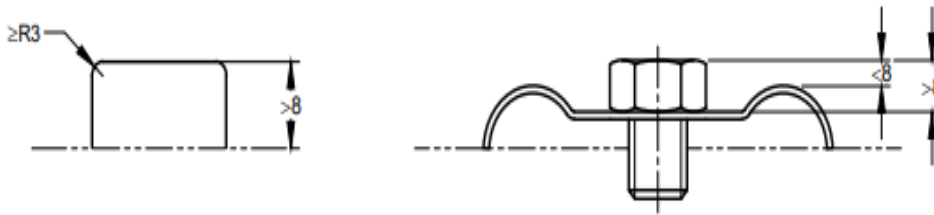
FIG. 3B EXAMPLE OF PERMISSIBLE PROTRUDING PARTS
