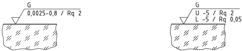
a) Indication for matt surface texture with Rq \leq 2 mm over a spatial band of 0,002 5 mm to 0,8 mm
