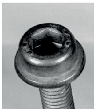
a) Zinc-nickel after 72 h NSS testing
