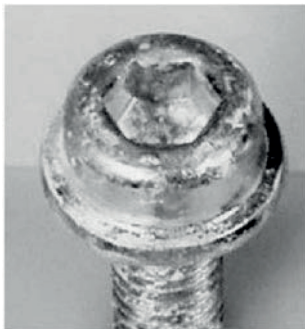
a) White corrosion of iridescent passivated zinc layer after 240 h NSS testing
