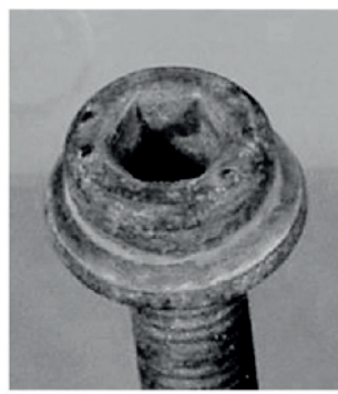
b) Zinc-nickel after 1 000 h NSS testing
