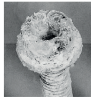
b) Severe white corrosion of iridescent passivated zinc layer after 480 h NSS testing
