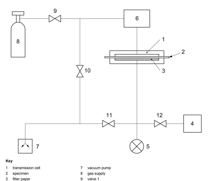
Figure A.1 — Example of gas transmission rate measurement apparatus using a pressure sensor
