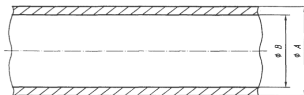
FIG. 7 WIRELINE CORE BARREL INNER TUBE (LOWER END)
