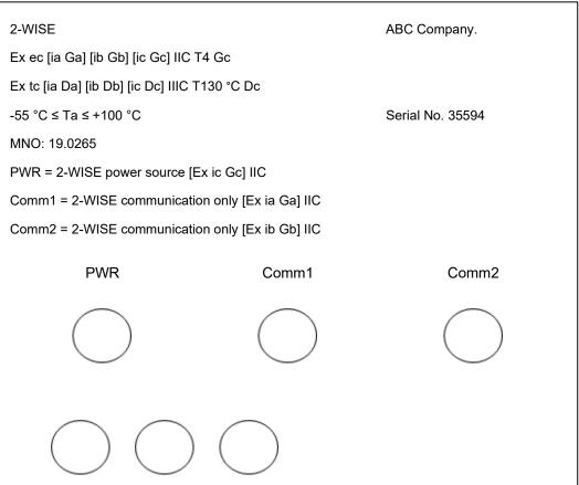
f) 2-WISE device with 2-WISE auxiliary device ports and a power load port
