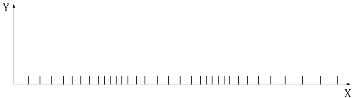
Figure A.4 — Periodic samples — CTVV — Periodic samples taken at fixed flow-intervals (volume-dependent) or CTVV sampling
