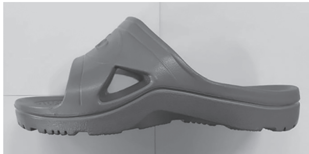
Figure B.1 — Example of homogeneous test sample
