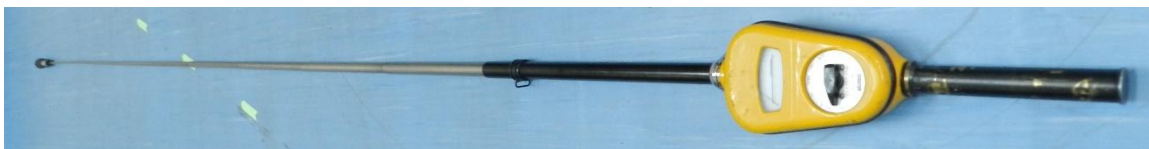
FIG. 2 COMMONLY USED DETECTOR (TELETECTOR) IN INDUSTRIAL RADIOMETRY
