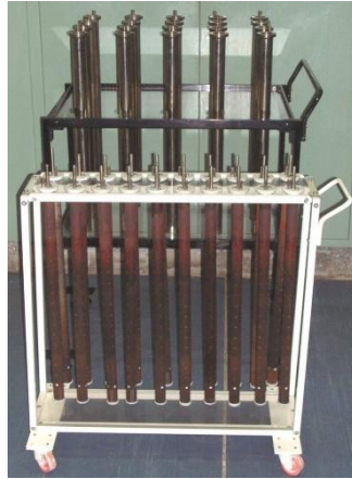
FIG. 2 ANODE AND DEVELOPED CATHODE ELECTROLYTIC CELL
