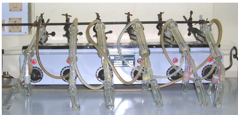
FIG. 5 NEUTRALISATION SETUP FOR SAMPLES POST ELECTROLYSIS
