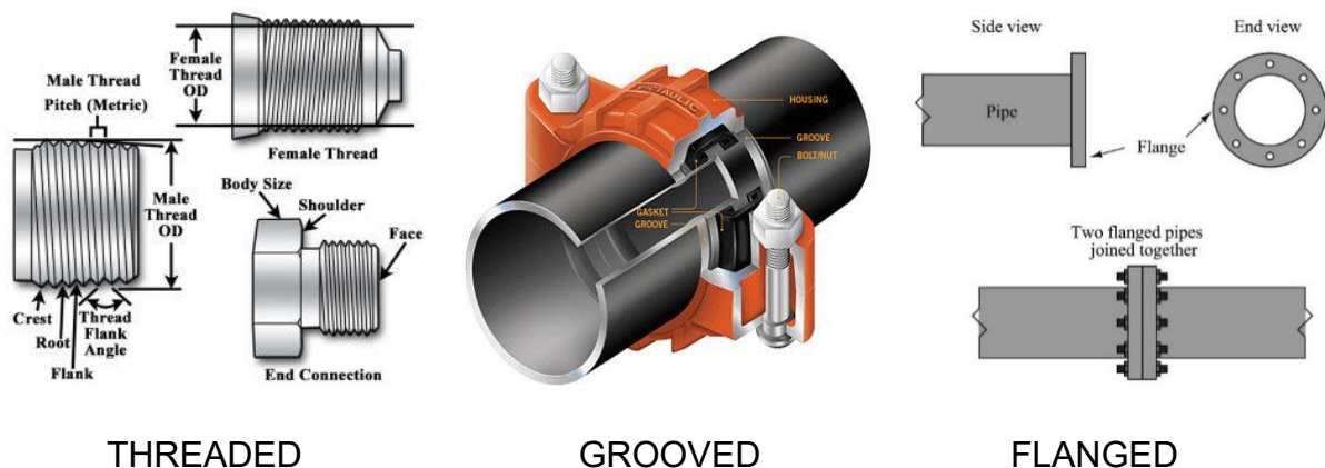
FIG. 14 PIPING CONNECTION METHODS
