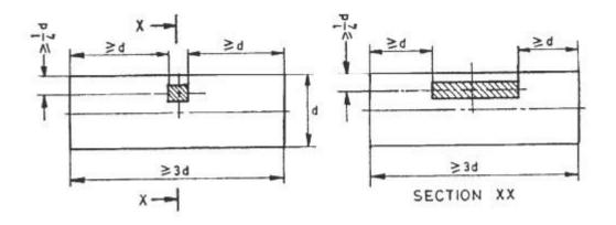
*d* is the thickness of the ruling section. FIG. 1 POSITION OF THE TEST PIECE AND SIZE OF THE SAMPLE
