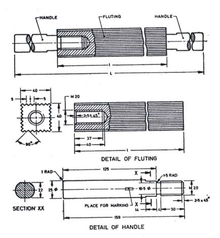
FIG. 1 DETAIL OF FLUTING AND HANDLE
