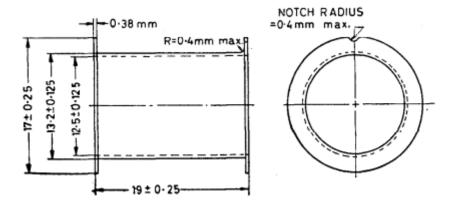
All dimensions in millimetres. FIG. 1 SKETCH OF THE SPOOL
