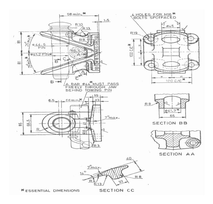
All dimensions in millimetres. FIG. 1 TOWING JAW FOR TRAILERS UPTO 16 TONNES
