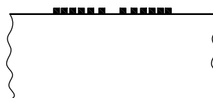
e) Diffractive binary-optic microlens
