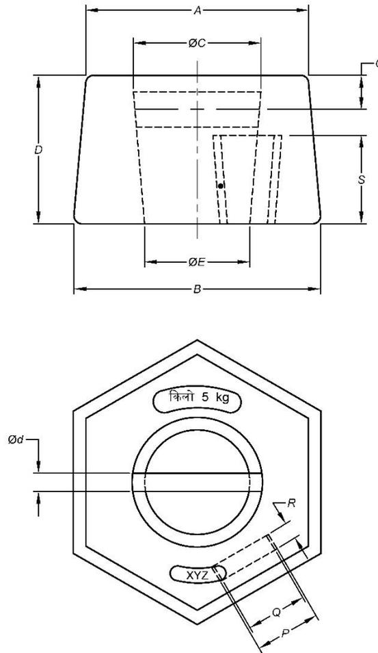
FIG. 1 CAST IRON WEIGHT WITH CAST-IN HANDLE
