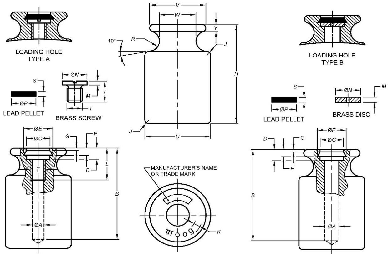
FIG. 3 CYLINDRICAL, KNOB TYPE WEIGHTS
