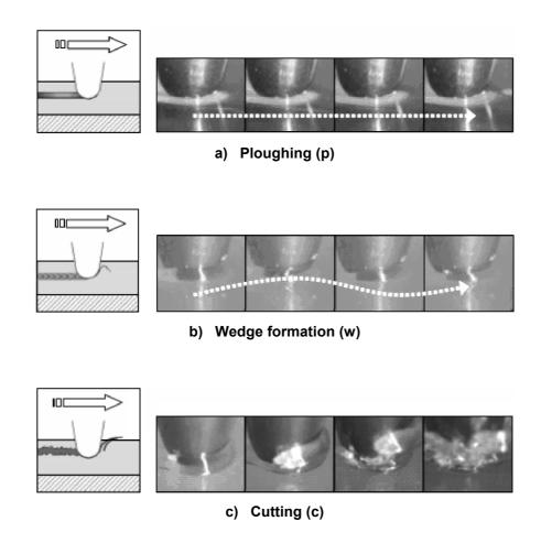
Figure A.1 — Photographs of different types of scratch behaviour as defined in 3.7.1 to 3.7.3
