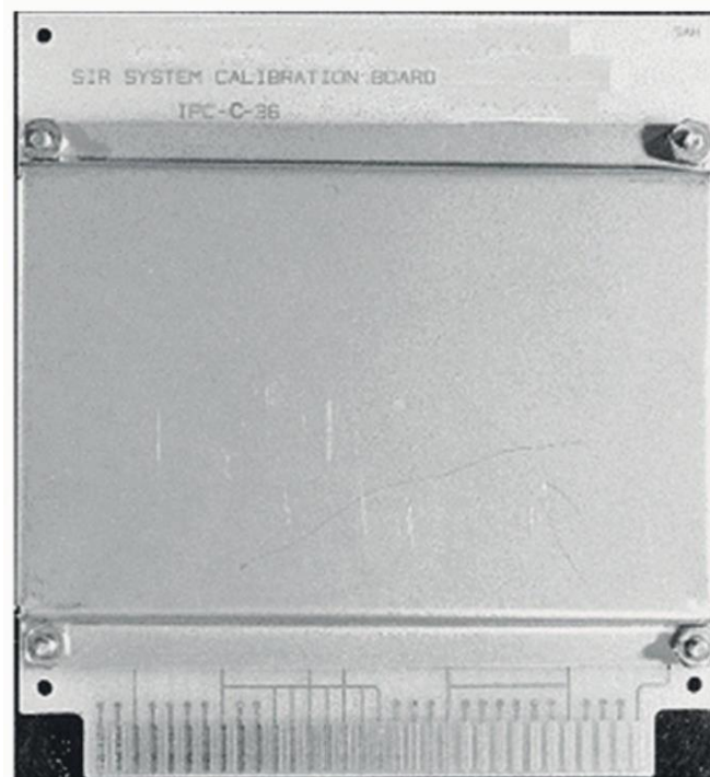
FIG. 12 RESISTOR VERIFICATION BOARD WITH PROTECTIVE COVER
