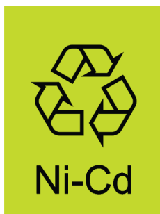
Figure 7 – Example of marking with recycling symbol for nickel cadmium batteries
