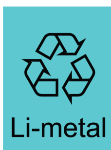
Figure 10 – Example of marking with recycling symbol for lithium metal batteries
