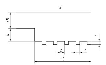
c) Detail of the clamping system (Z)
