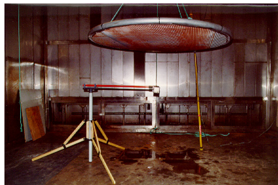
Figure F.1 – Test in the climatic chamber with the normal tripod (left) and the offset tripod (right) (photograph EDF R&D)
