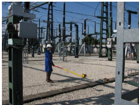
Figure 3 – Electric field measurement using a hand-held stick (photograph RTE)
