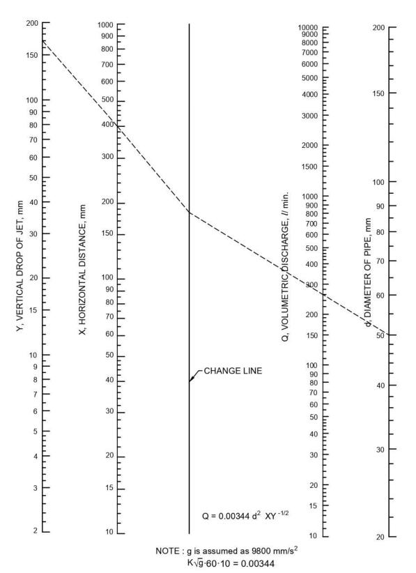
FIG. 2 NOMOGRAPH FOR SOLUTION ON JET CHARACTERISTICS OF FLOW
