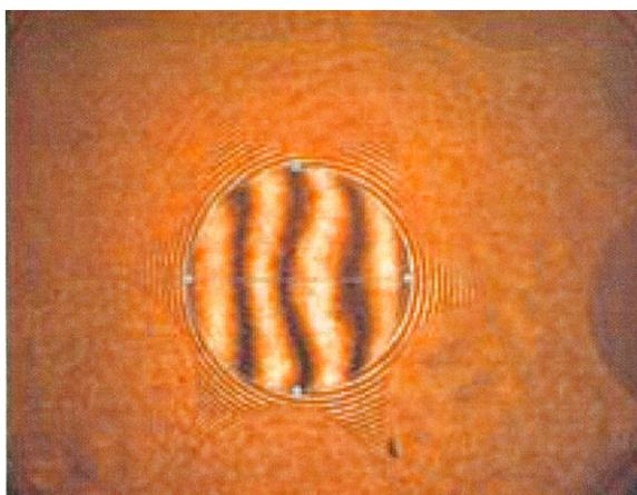
The interference fringes give a clear indication of spherical aberration.
