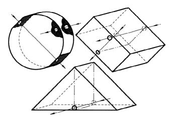
Figure 3 — Examples of test samples, including possible measuring points
