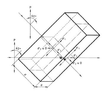
Figure 1 — Principal stresses shown in a rectangular plate
