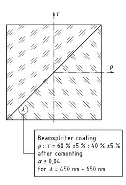
Figure 3 — Example of functional coating indication with optical characteristic specification
