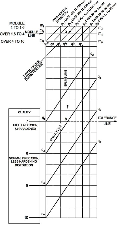
Table 12 Tolerance for Spline Tooth Thickness and Space Width
