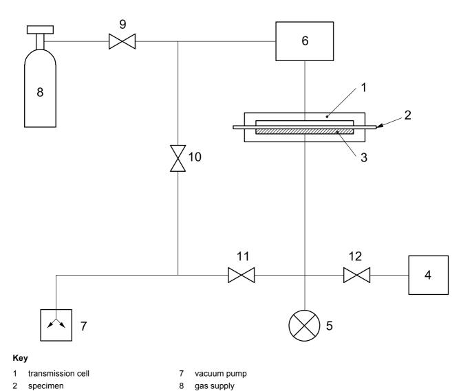
Figure A.1 — Example of gas transmission rate measurement apparatus using a pressure sensor
