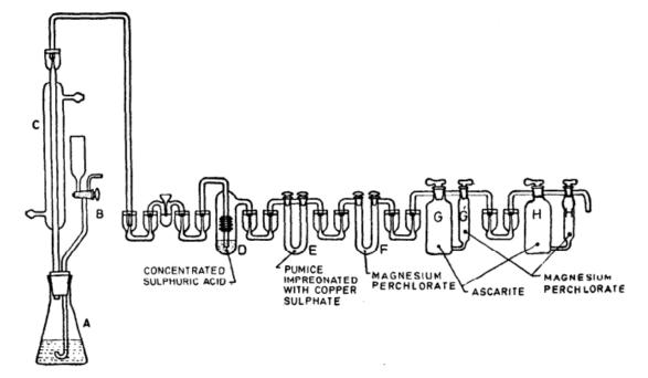
NOTE — Tubes are compactly arranged along the edge of 150 mm  $\times$  230 mm board which is supported 130 mm from the table-top upon a tripod base.
