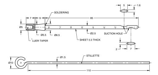
All dimensions in millimetres. FIG.1 CANNULA, BRAIN
