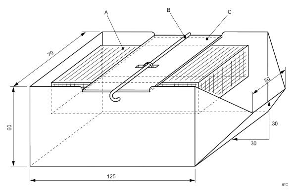
This displacement block has a volume of 140 ml  $\pm\,5$  ml and a mass of 200 g  $\pm\,10$  g.
