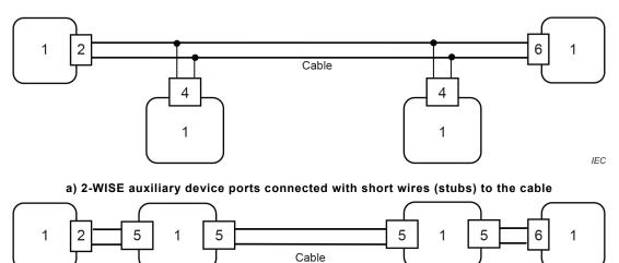
b) 2-WISE auxiliary device ports connected via a series connection in the cable
