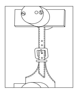
FIG. 4 ILLUSTRATION DIAGRAM FOR ATTACHMENT STRENGTH OF STRAP, BUCKLE, D-RING, VELCRO
