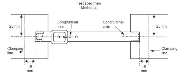
FIG. 6 CUTTING OF WHOLE TEST ASSEMBLY–BUCKLE ATTACHED TO SANDAL UPPER VIA SEPARATE BUCKLE LOOP
