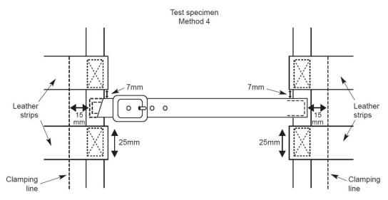
FIG. 8 CUTTING OF TEST SPECIMEN—WHOLE ASSEMBLY WITH SEWN ON STRIPS-BUCKLE STRAP ATTACHED TO SLING BACK STRAP
