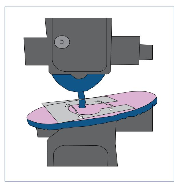
FIG. 2 ILLUSTRATION DIAGRAM FOR CLAMPING OF TOE POST STRAP IN THE TENSILE MACHINE
