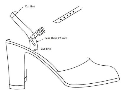
FIG. 7 CUTTING OF TEST ASSEMBLY-BUCKLE STRAP ATTACHED TO SLING-BACK STRAP
