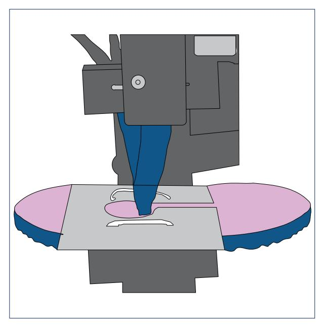
FIG. 3 ILLUSTRATION DIAGRAM FOR CLAMPING OF REAR STRAP IN THE TENSILE MACHINE
