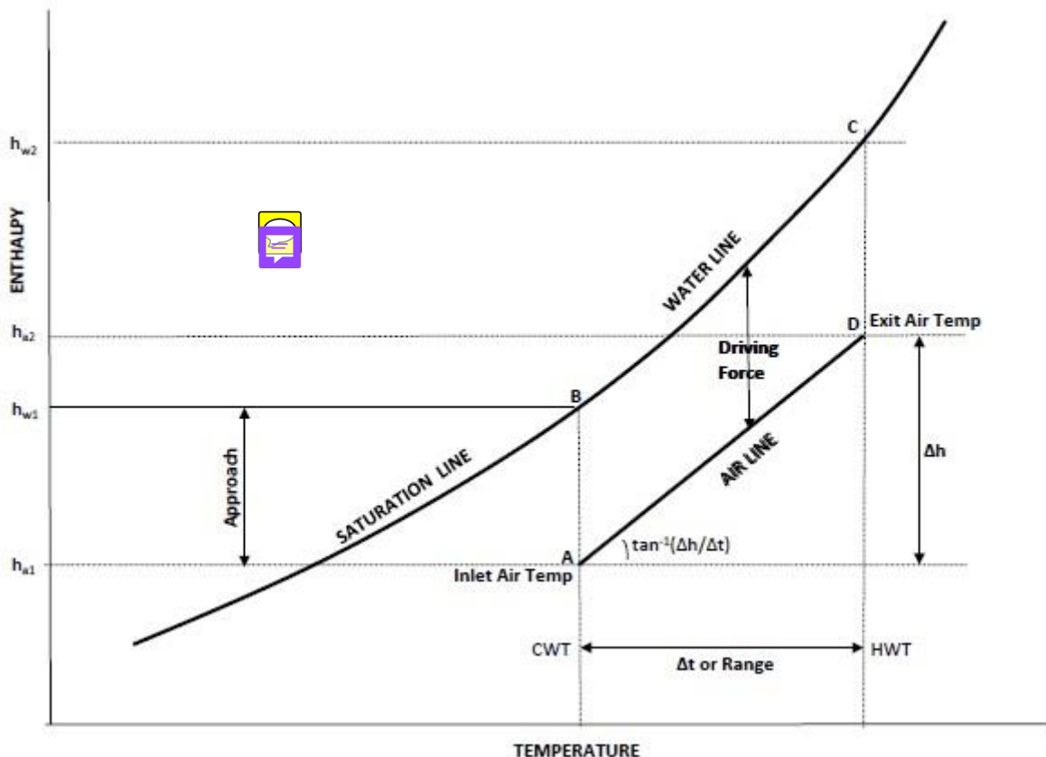
FIG. 12 HEAT TRANSFER DIAGRAM
