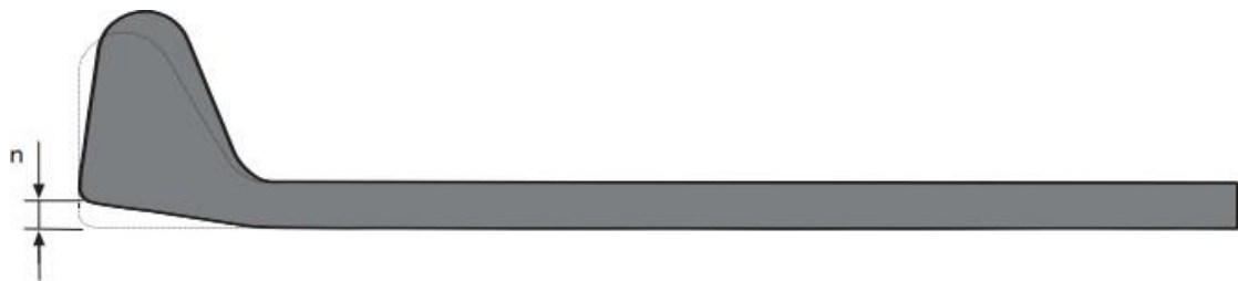
FIG. 5 BULB FLATNESS TOLERANCE OF BULB FLAT
