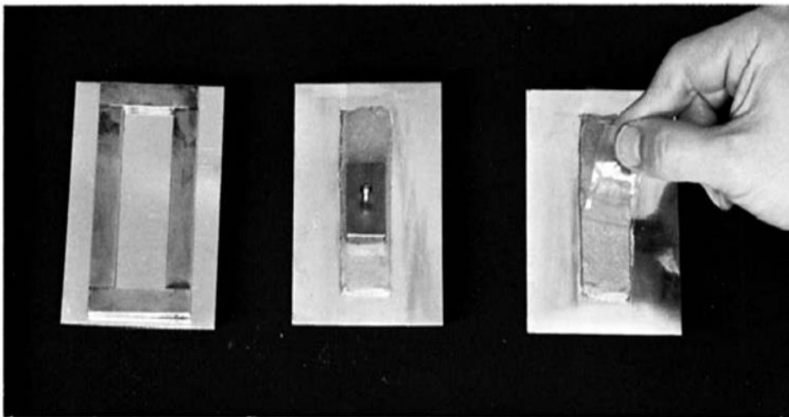
FIG. 5 STAGES IN THE TACK-FREE TIME TEST PROCEDURE
