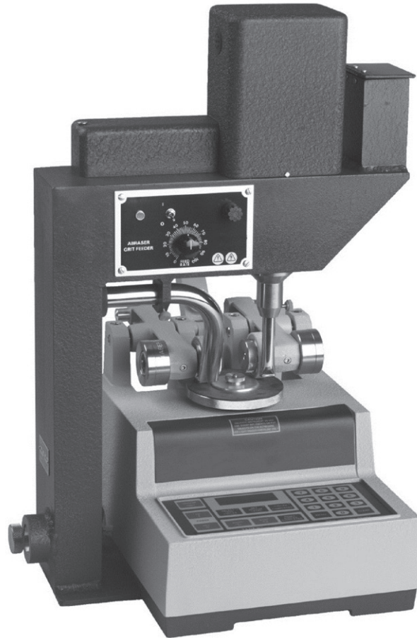
Figure 2 — Example of a Taber® Abraser with Grit Feeder 3)
