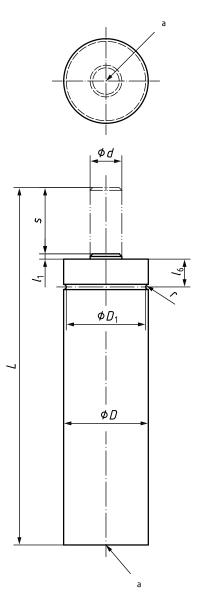
The general tolerance shall be ISO 2768-m according to ISO 2768-1.
