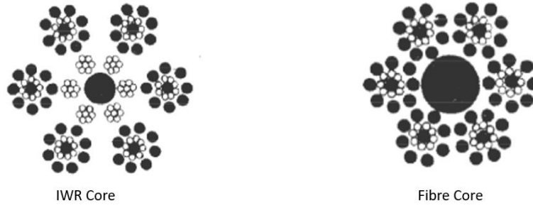
FIG. 1 6 \times 8 (8/f) COMBINATION WIRE ROPES
