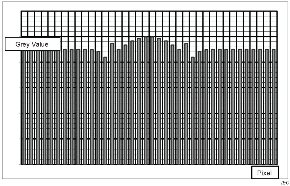
Figure CC.9 – Grey value profile over a sphere by low contrast
