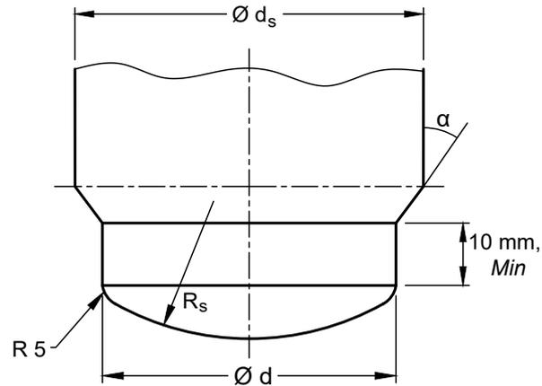
8A TYPE  $d_{25}$  ( FOR STRIKERS OF MASS 0.25 kg AND 0.5 kg )
