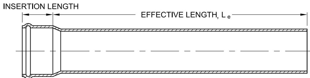
2B SOCKETED PIPE FOR ELASTOMERIC SEALING RING JOINT
