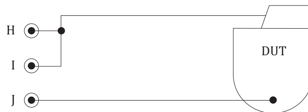
Figure 14 — Connection to a single-channel unipolar device
