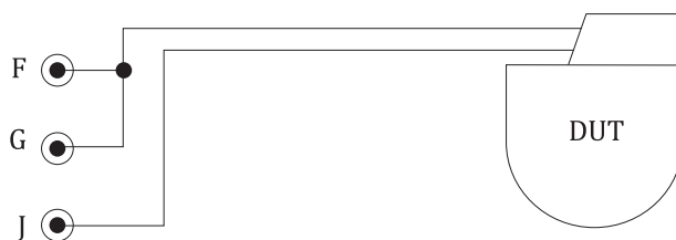
Figure 6 — Differential mode connection to single-channel bipolar device
