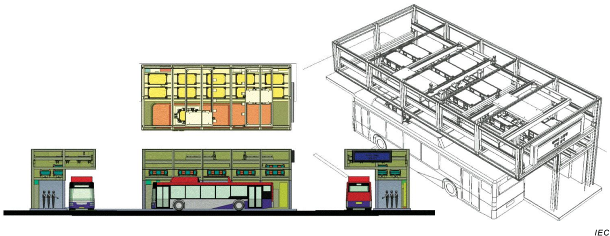
Figure B.2 – Automatic top-swapping station layout
