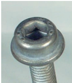
a) White haze on zinc-nickel after 72 h NSS testing
