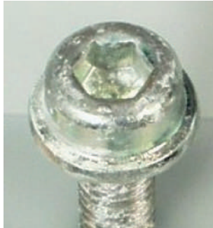
a) White corrosion of iridescent passivated zinc layer after 240 h NSS testing
