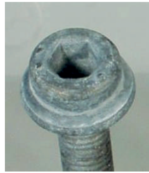
b) White haze on zinc-nickel after 1 000 h NSS testing
