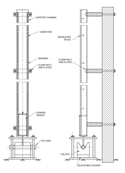
FIG. 7 IMPACT TESTING MACHINE
