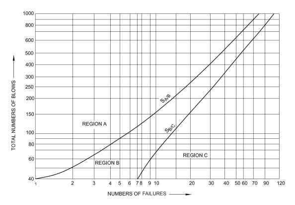
Fig. 9 Number of Test Pieces for 10 Percent Tir (at 90 Percent Confidence Level)
