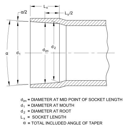
FIG. 3 SOCKET DIMENSIONS FOR SOLVENT CEMENT JOINTS
