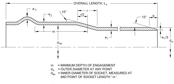
Fig. 4 Socket for use with Elastomeric Sealing Rings
