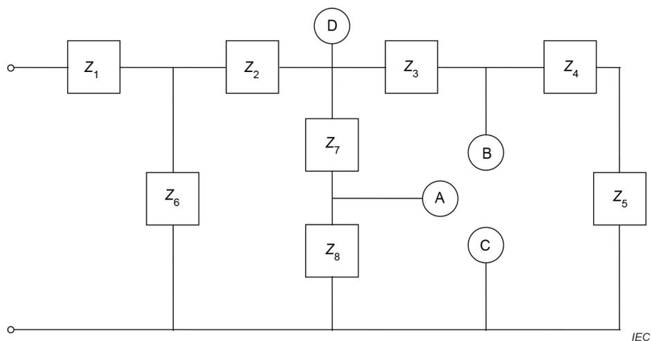
D is a point farthest from the supply source where the maximum power delivered to external load exceeds 15 W.
