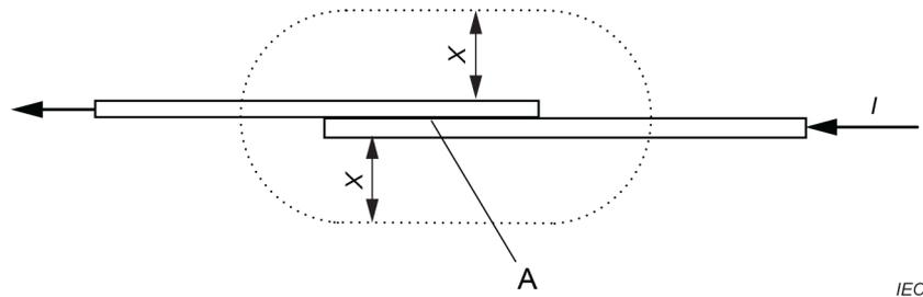
"Within a distance of 3 mm" means falling within the dotted boundary formed by the cylinder with hemispherical ends, as shown in the above drawing.
