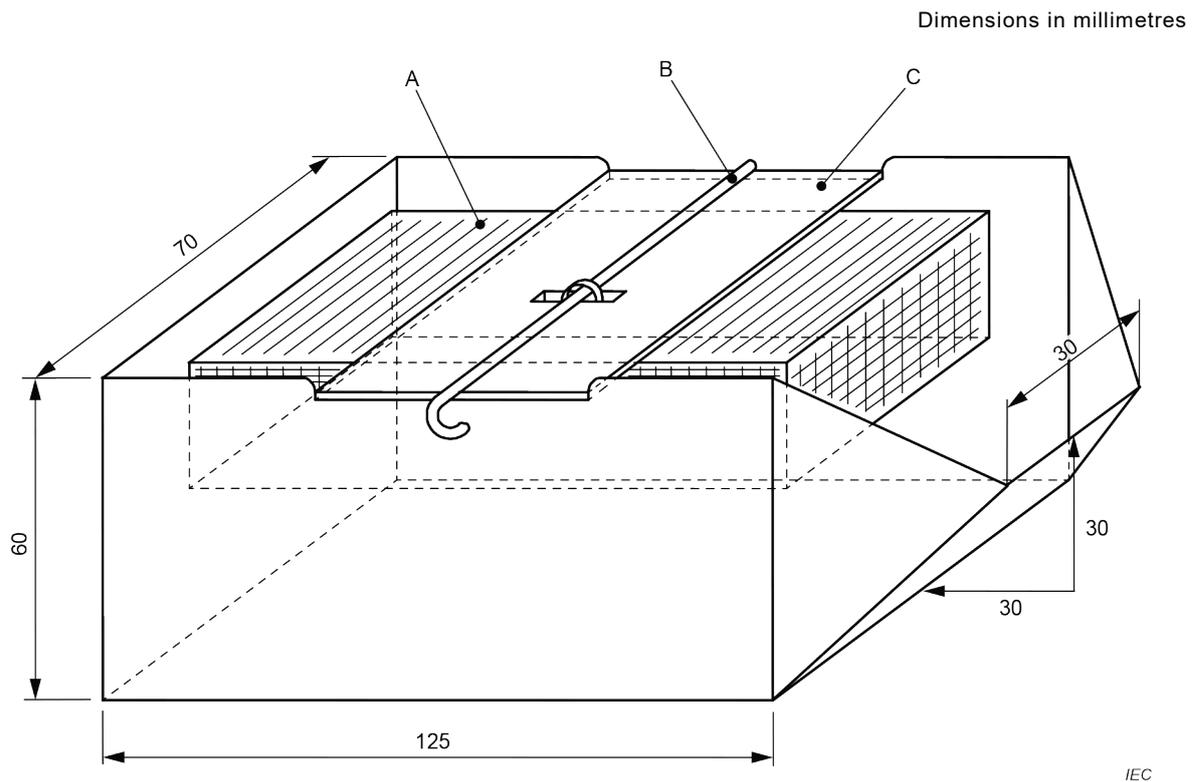
This displacement block has a volume of  $140 \text{ ml} \pm 5 \text{ ml}$  and a mass of  $200 \text{ g} \pm 10 \text{ g}$ .
